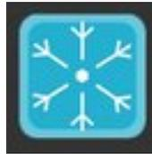
If the machine's coolers started for cooling, this indicator will be flash.
