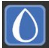
If the machine's humidifiers started for moisturing, this indicator will be flash.
